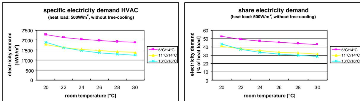
Figure 4-9: Specific electricity demand (kWh per  $m^2$  and per year, and percentage of heat load) for cooling and ventilation without free cooling depending on the computer room air temperature and the cold water and cooling air temperature (Altenburger, 2001).
