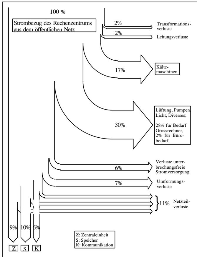
The split of the electricity consumption can be determined in a first order approximation by a measurement of the power-flow (see figure):
