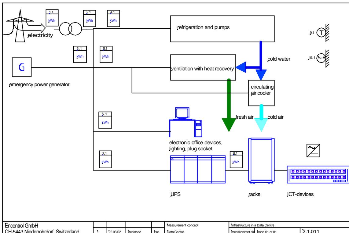
Figure 4-3: Measurement concept for data centres (see Table 4-1)
