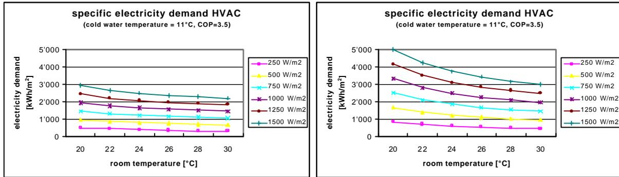
Figure 4-8: Specific electricity demand (kWh per  $m^2$ ) for cooling and ventilation depending on the computer room air temperature, air flow velocity and fan efficiency (Altenburger, 2001). Left: Air velocity 1.5m/s, fan efficiency 65%. Right: Air velocity 3m/s, fan efficiency 55%.
